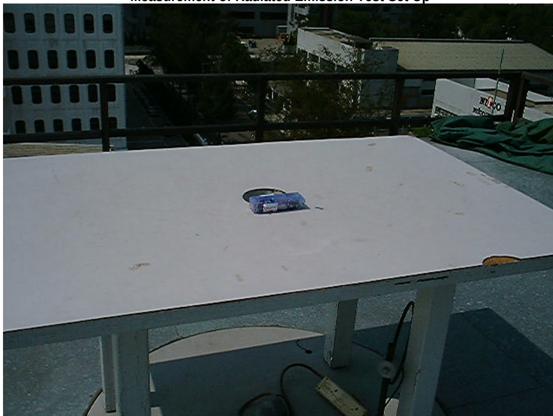
Measurement of Radiated Emission Test Set Up
