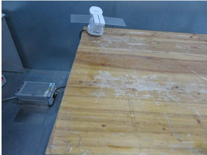
Conducted Emissions at Mains Terminals
