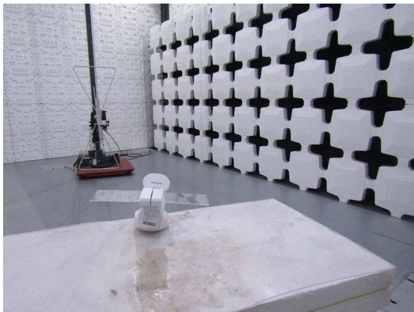
Radiated Emissions below 1GHz
