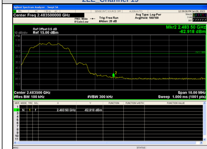
Out Of Band Emission 2LE_Channel 39
