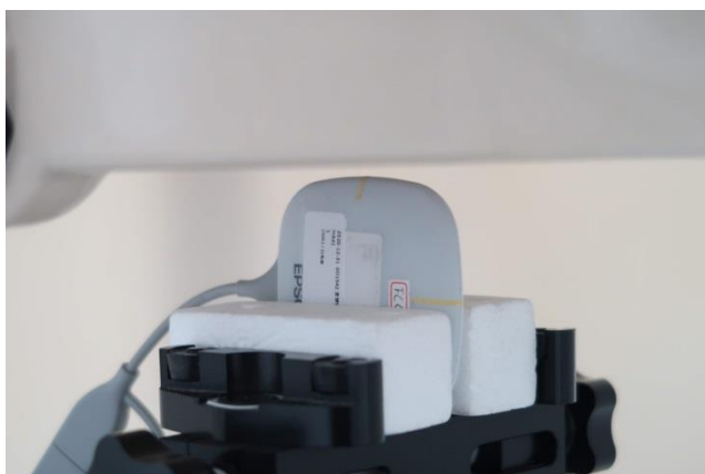
Vertical Back, Test Separation 5 mm
