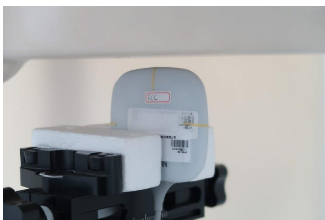
Tip Mode, Test Separation 5 mm
