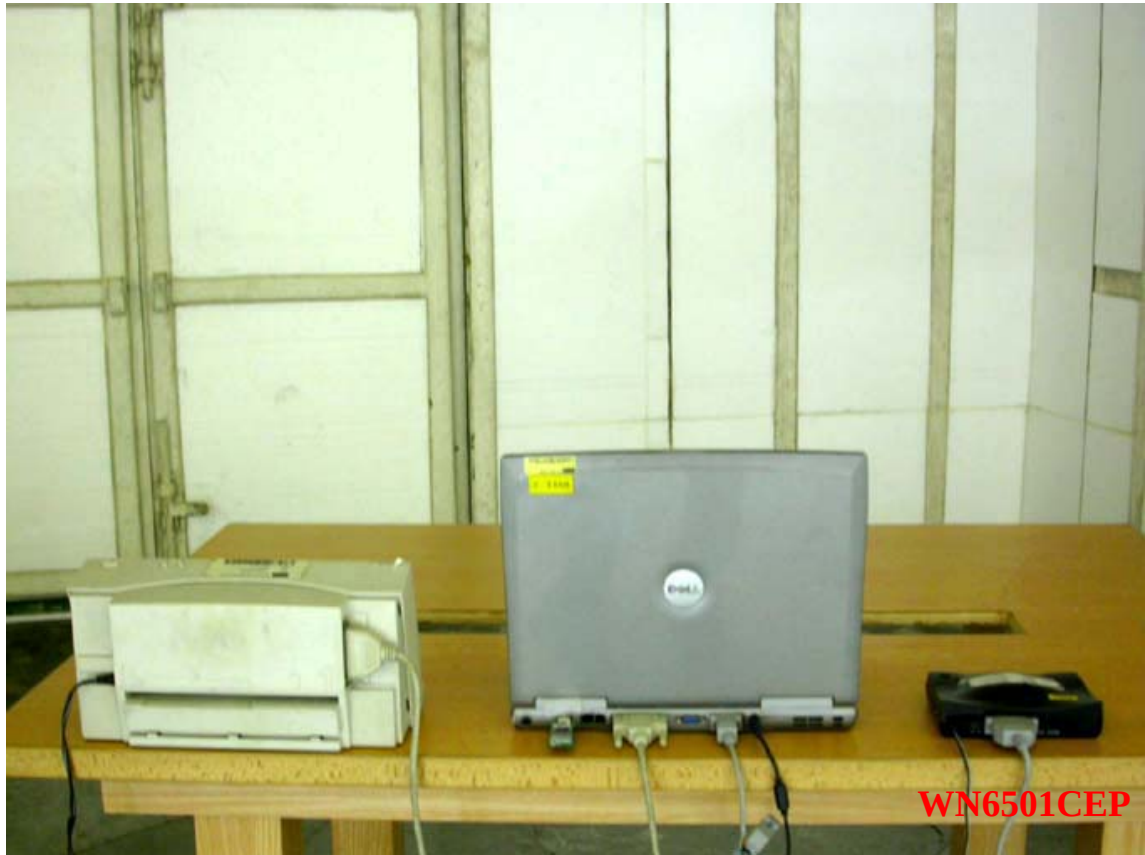
Photo 3: Radiated Emission Test Set-up
