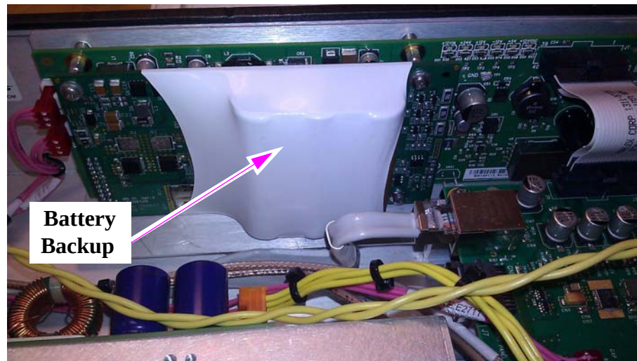
Figure 5-10 Battery Backup (UPS) Location
