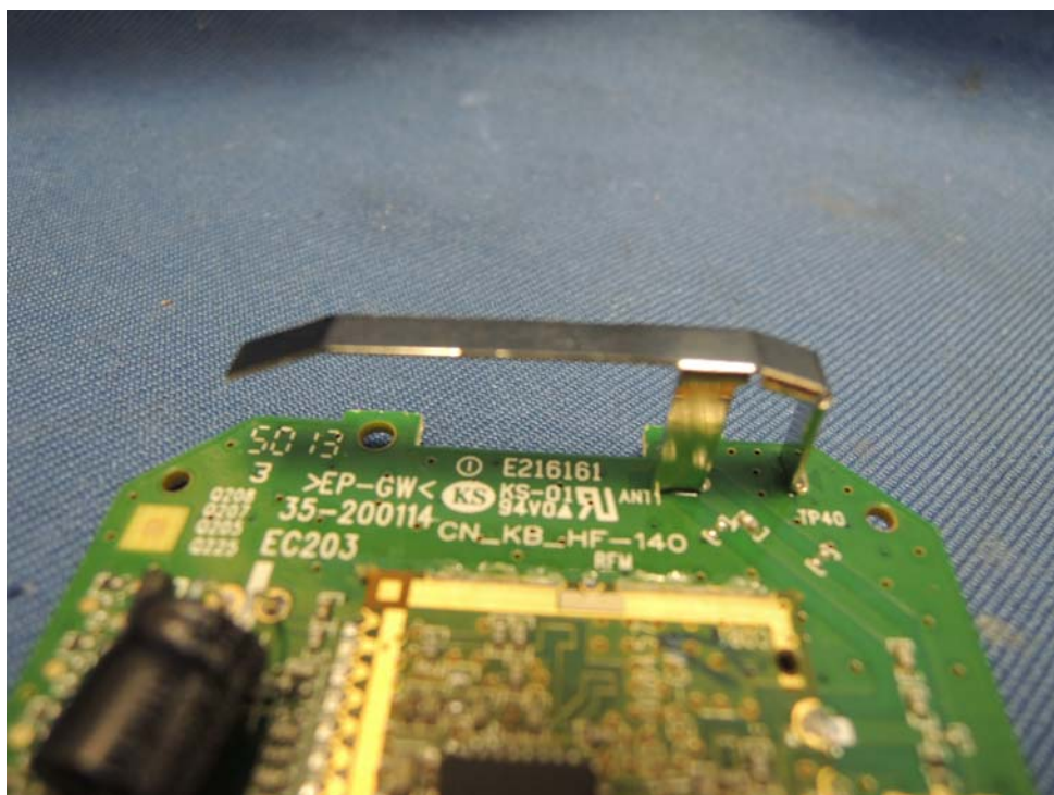
Parent Unit Main PCB Antenna
