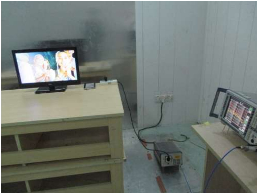
FCC RADIATED EMISSION TEST SETUP
