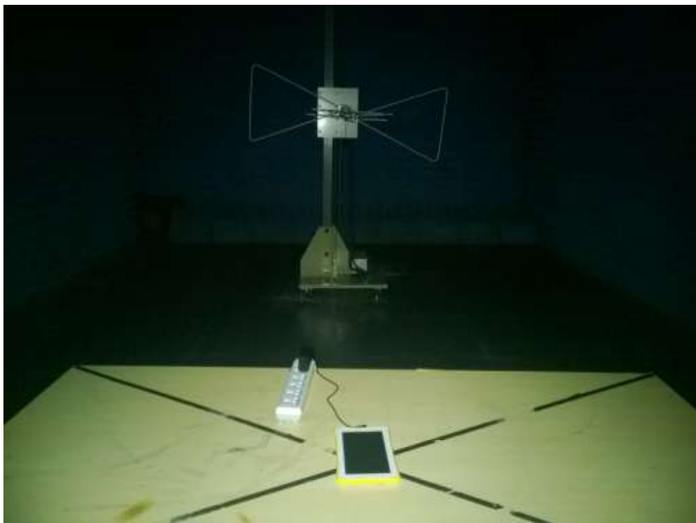
FCC RADIATED EMISSION TEST SETUP
