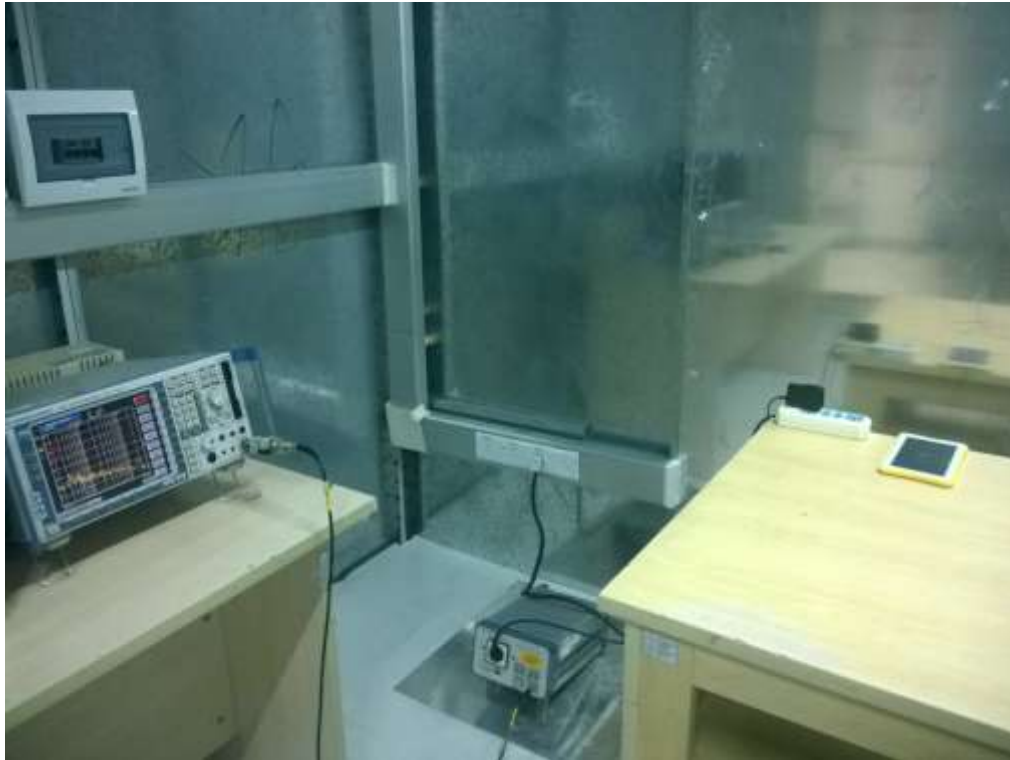
FCC RADIATED EMISSION TEST SETUP
