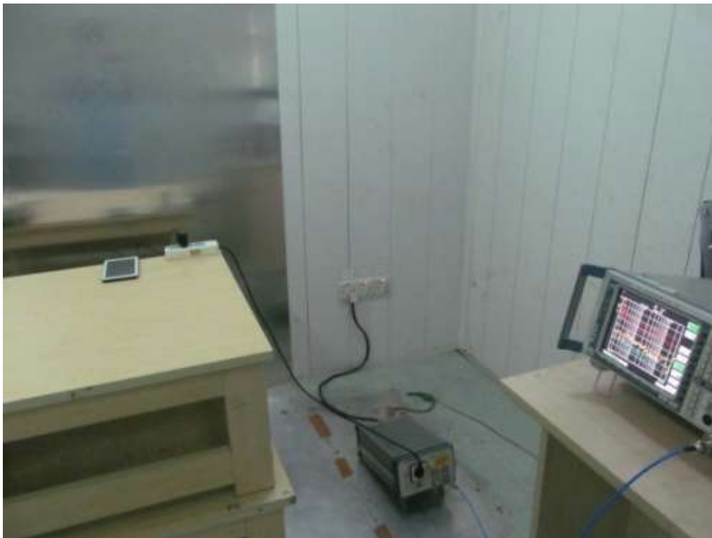
FCC LINE CONDUCTED EMISSION TEST SETUP
