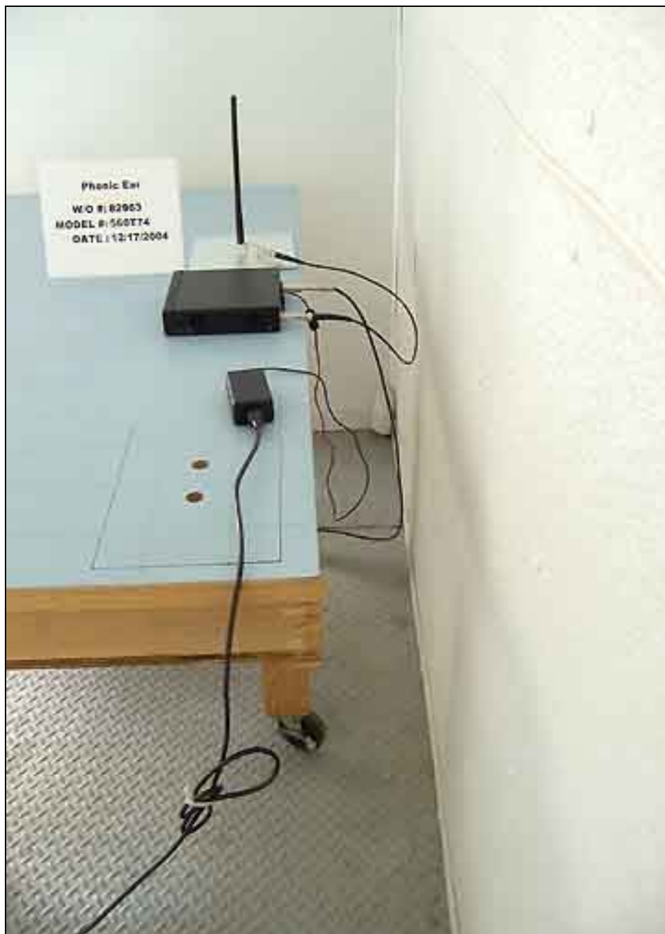
Mains Conducted Emissions - Side View
