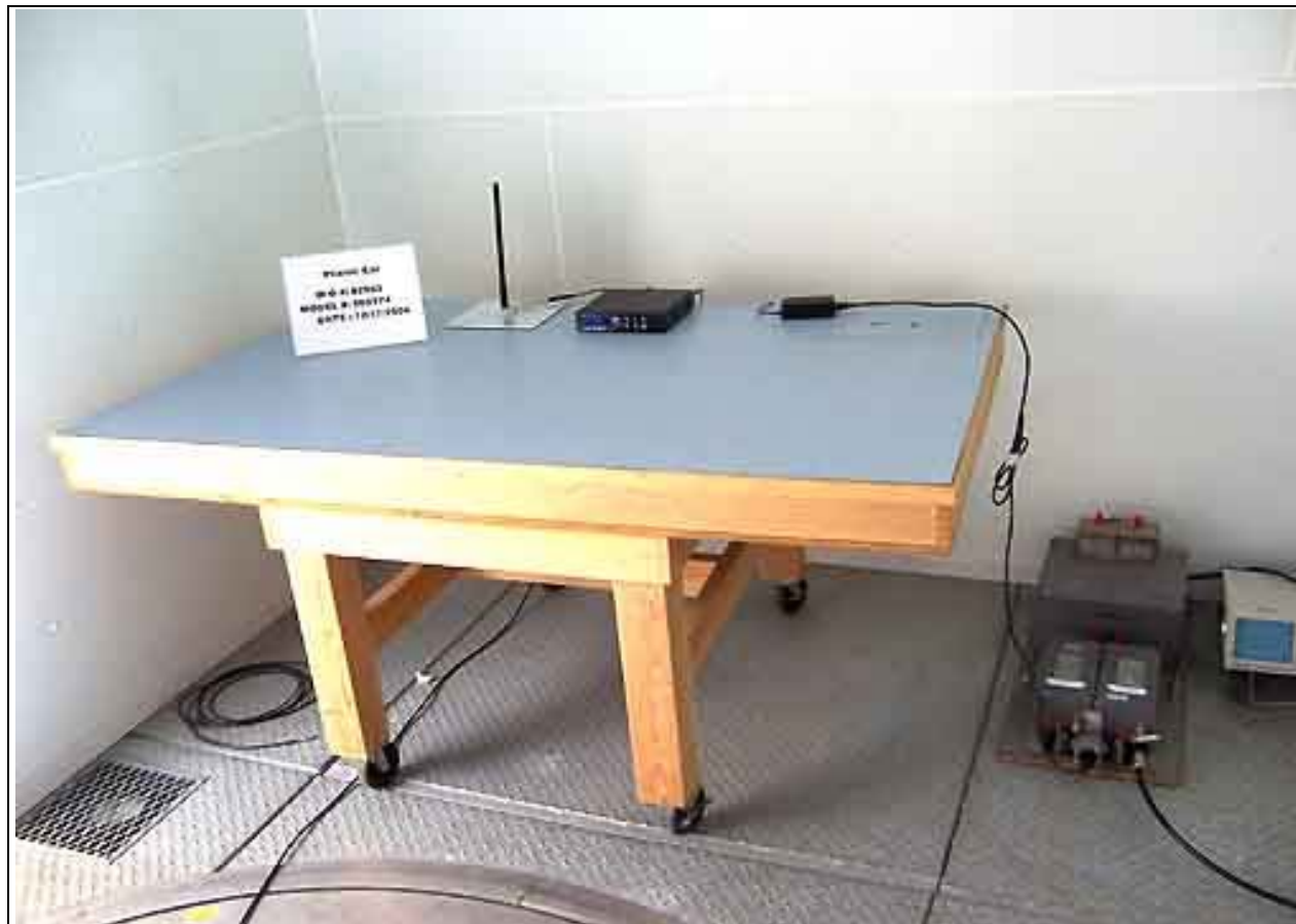
Mains Conducted Emissions - Front View
