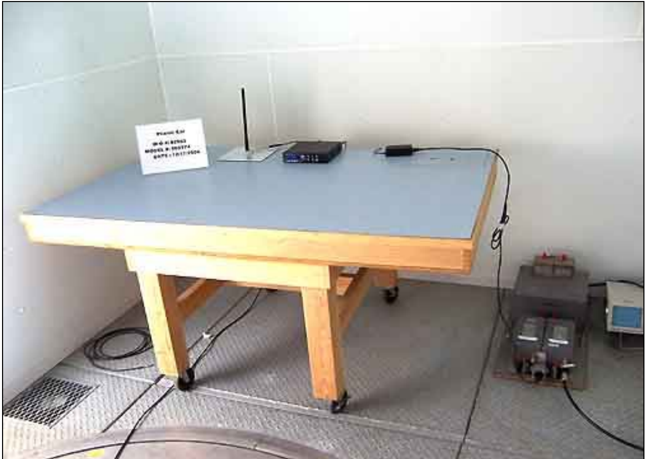
Mains Conducted Emissions - Front View
