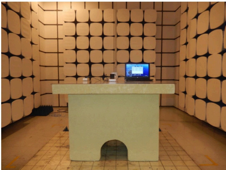
Photograph 2: Set-up for Spurious Emissions (above 1GHz)
