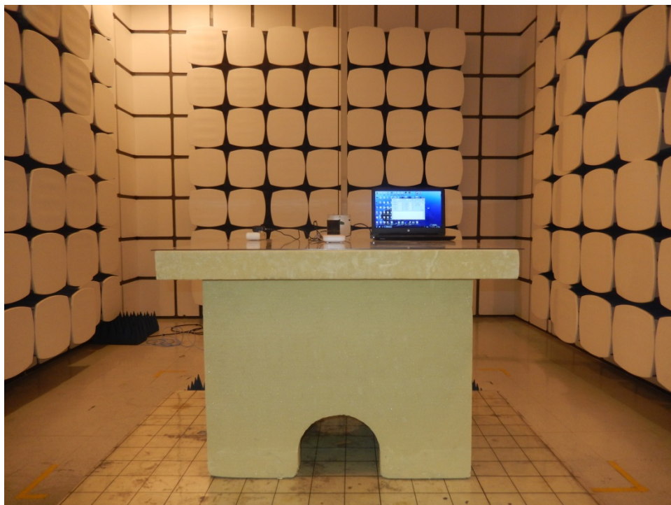
Photograph 2: Set-up for Spurious Emissions (above 1GHz)
