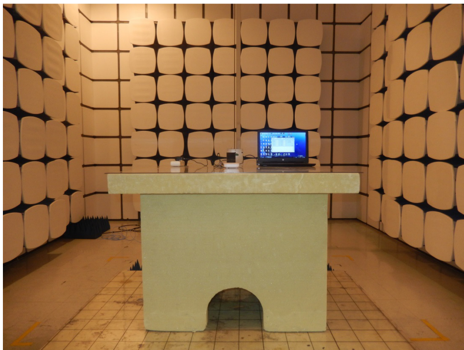
Photograph 2: Set-up for Spurious Emissions (above 1GHz)
