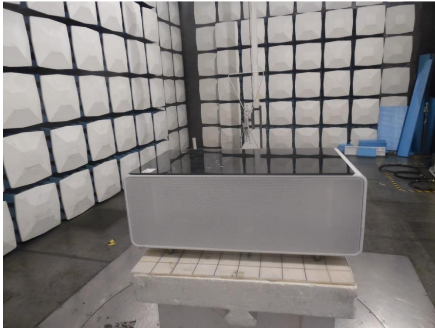
Photograph 2: Set-up for Spurious Emissions (above 1GHz)
