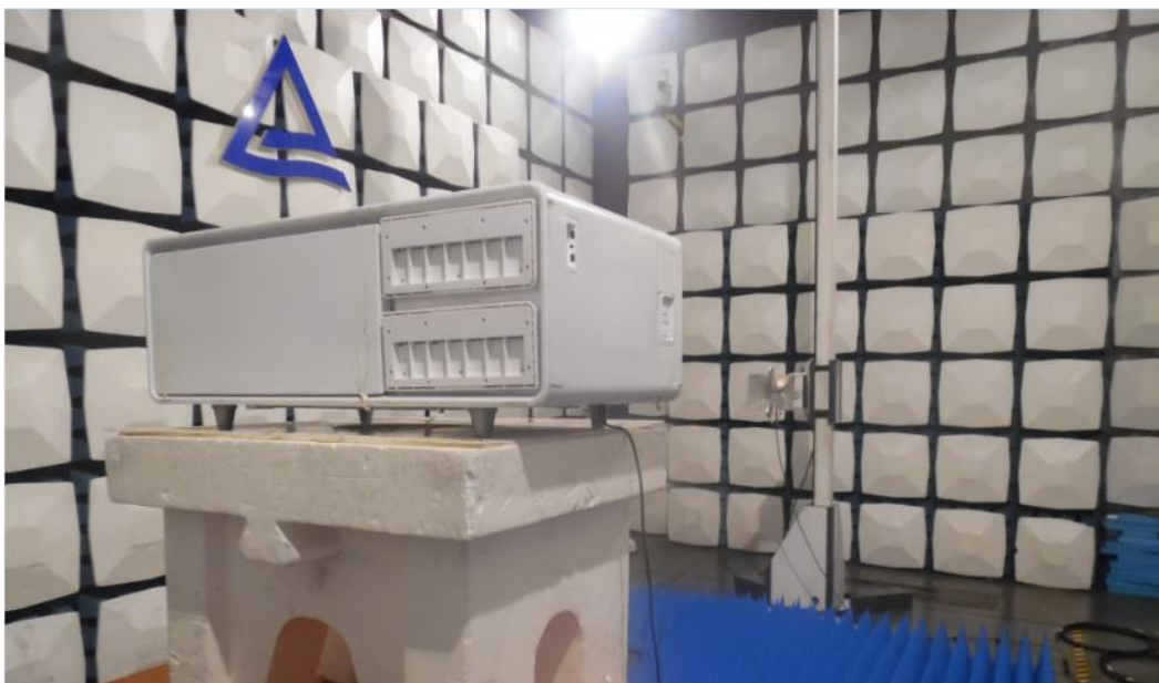
Photograph 2: Set-up for Spurious Emissions (above 1GHz)
