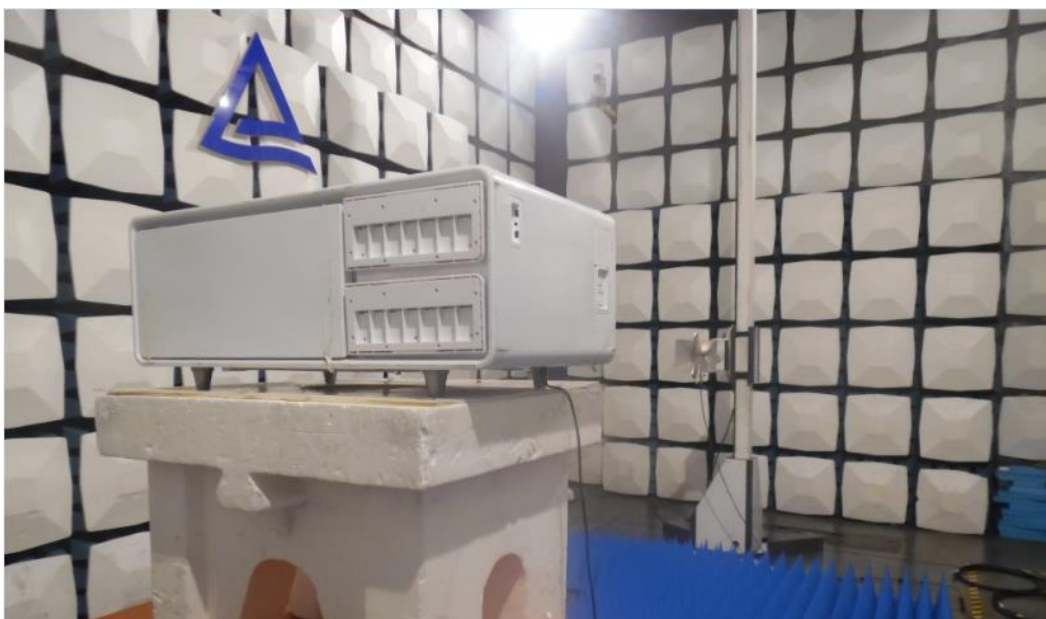
Photograph 2: Set-up for Spurious Emissions (above 1GHz)
