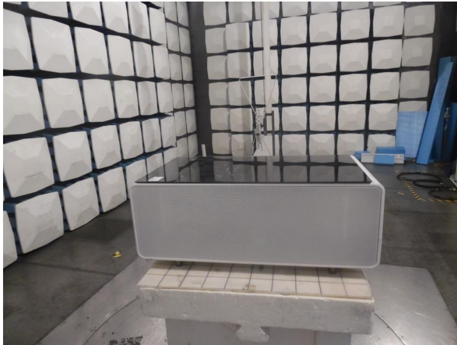
Photograph 2: Set-up for Spurious Emissions (above 1GHz)
