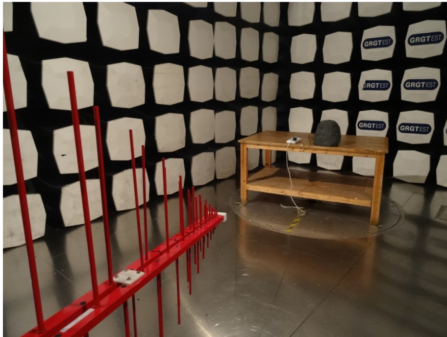
Photograph 2: Set-up for Spurious Emissions (above 1GHz)
