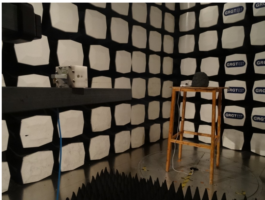
Photograph 2: Set-up for Spurious Emissions (above 1GHz)
