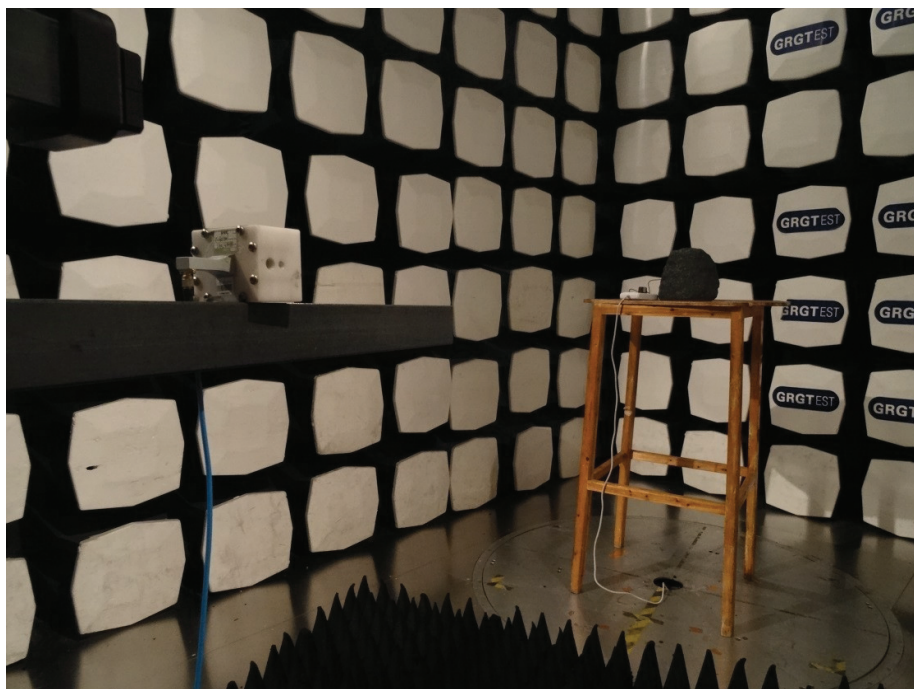
Photograph 2: Set-up for Spurious Emissions (above 1GHz)
