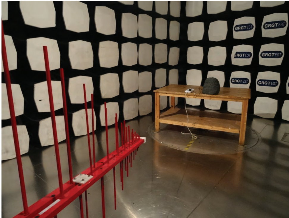
Photograph 2: Set-up for Spurious Emissions (above 1GHz)
