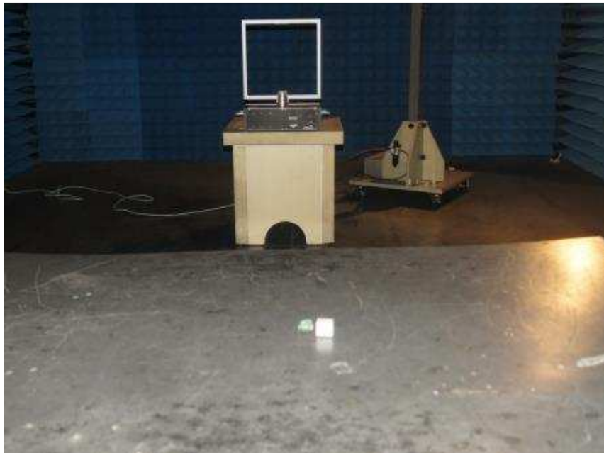
Photograph 2: Set-up for Radiated Spurious Emissions (30MHz-1GHz)
