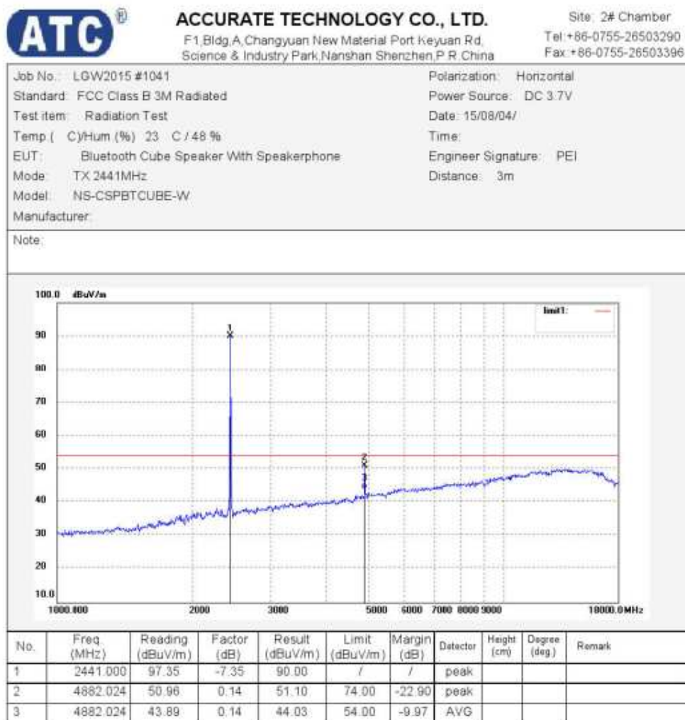
Figure 6: Test figure of Radiated Spurious Emissions (1GHz –25GHz), BDR (Mid)
