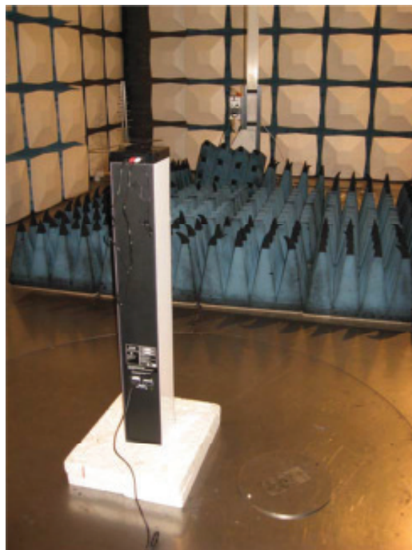
Photograph 3: Set-up for Radiation Measurement above 1GHz
