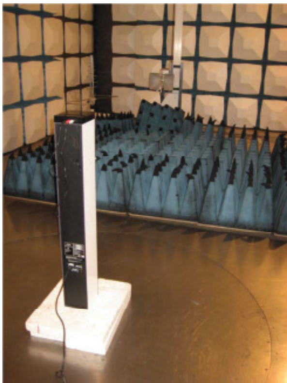
Photograph 3: Set-up for Radiation Measurement above 1GHz
