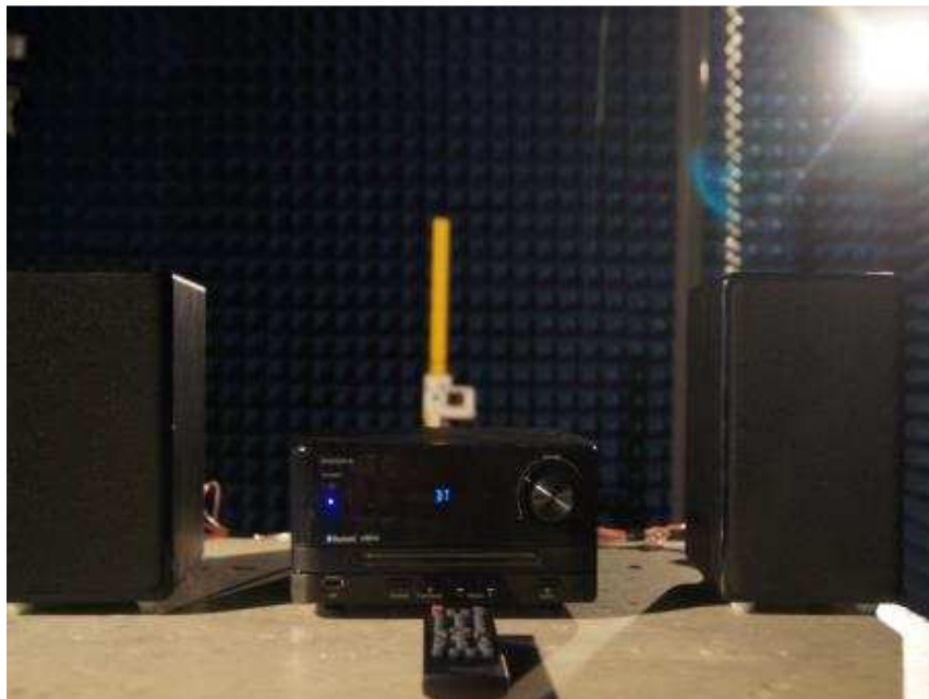
Photograph 4: Set-up for Radiated Spurious Emissions (18GHz ~ 26GHz)
