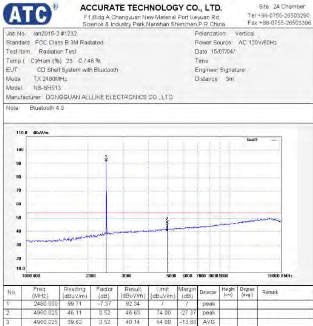
Figure 18: Test figure of Radiated Spurious Emissions (1GHz –25GHz), Low Energy (High)
