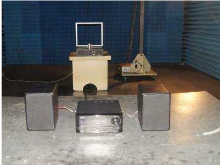
Photograph 2: Set-up for Radiated Spurious Emissions (30MHz-1GHz)
