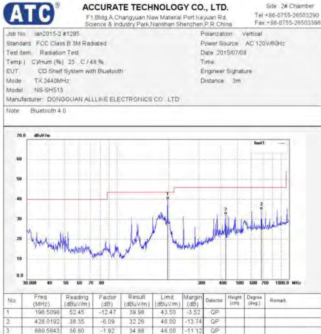
Figure 14: Test figure of Radiated Spurious Emissions (30MHz – 1GHz), Low Energy (Mid)
