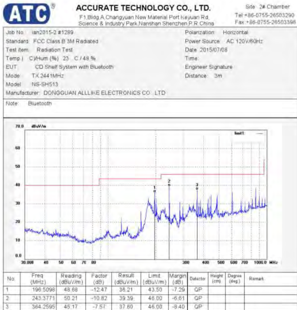
Figure 5: Test figure of Radiated Spurious Emissions (30MHz – 1GHz), BDR (Mid)
