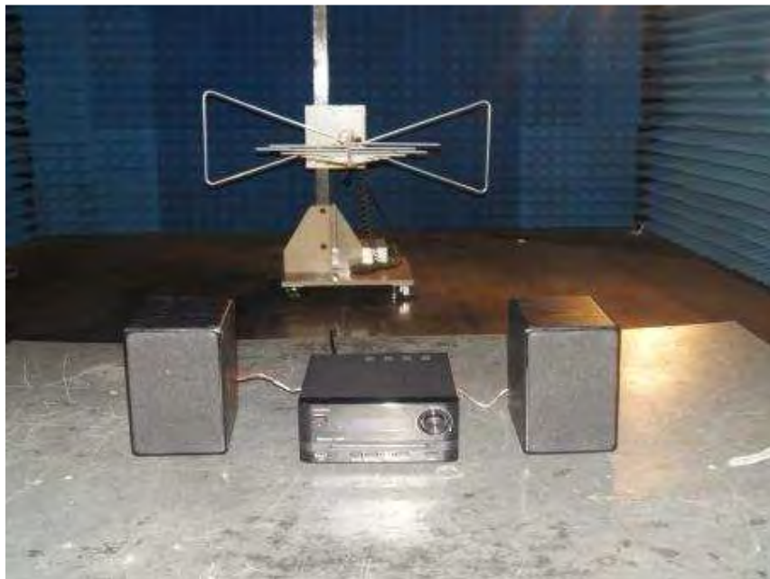
Photograph 2: Set-up for Radiated Spurious Emissions (30MHz-1GHz)
