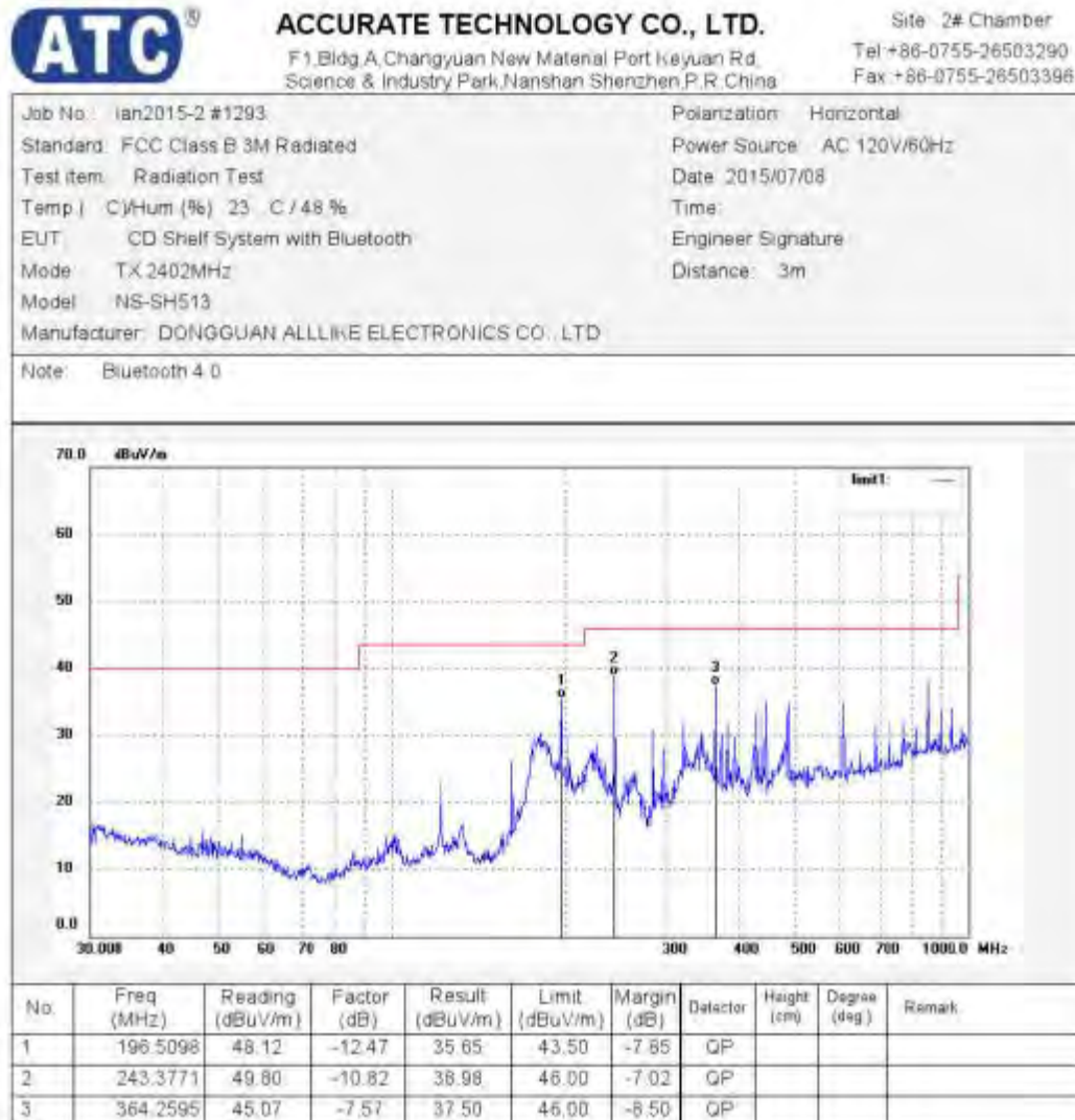
Figure 11: Test figure of Radiated Spurious Emissions (30MHz – 1GHz), Low Energy (Low)
