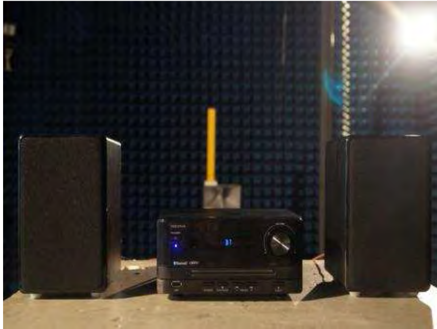
Photograph 4: Set-up for Radiated Spurious Emissions (18GHz ~ 26GHz)
