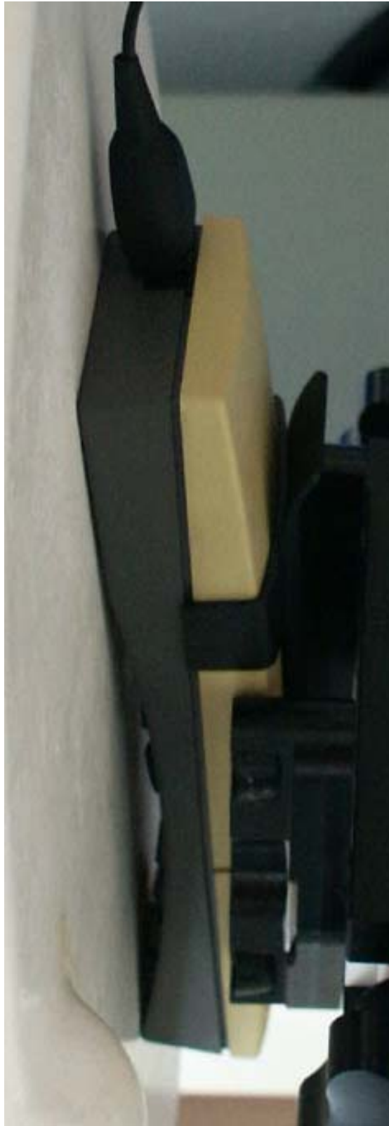
Fig. 24: Body worn configuration, belt clip with headset, display towards the phantom.
