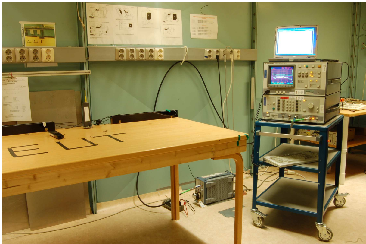
Power line Conducted Emissions Test
