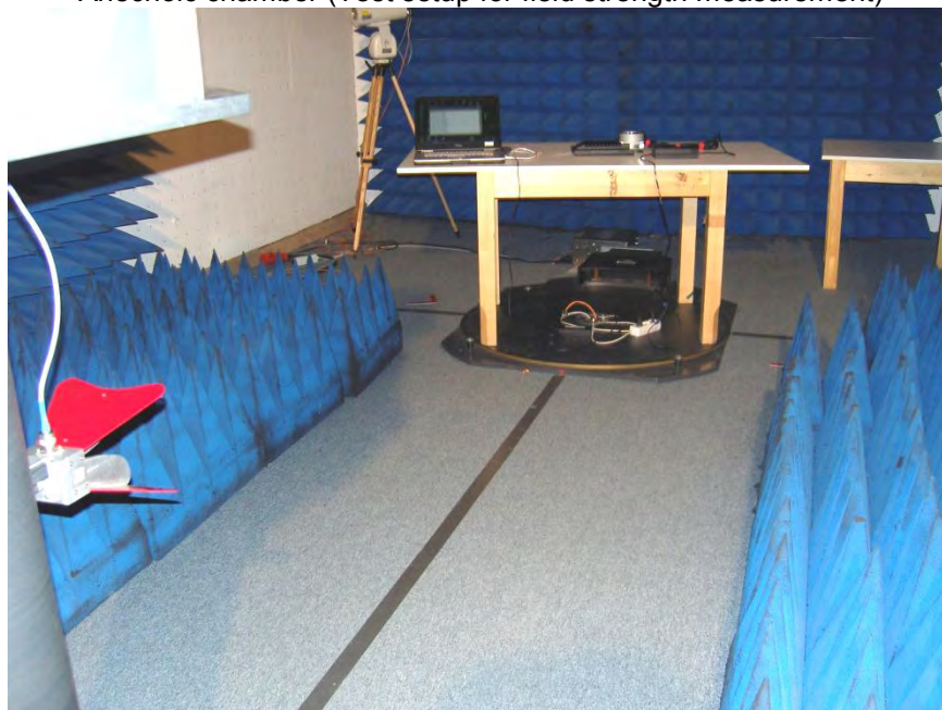
Anechoic chamber (Test setup for 18 GHz – 30 GHz)
