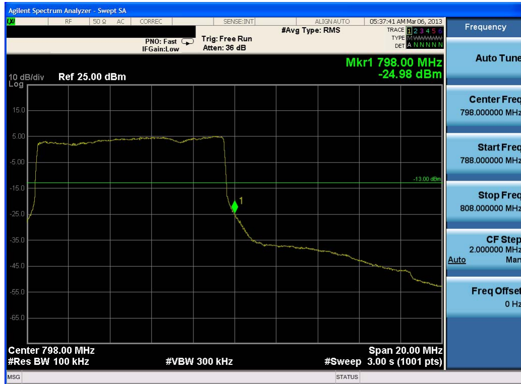
Plot 8-3. Upper Band Edge Plot (QPSK, 50RB)
