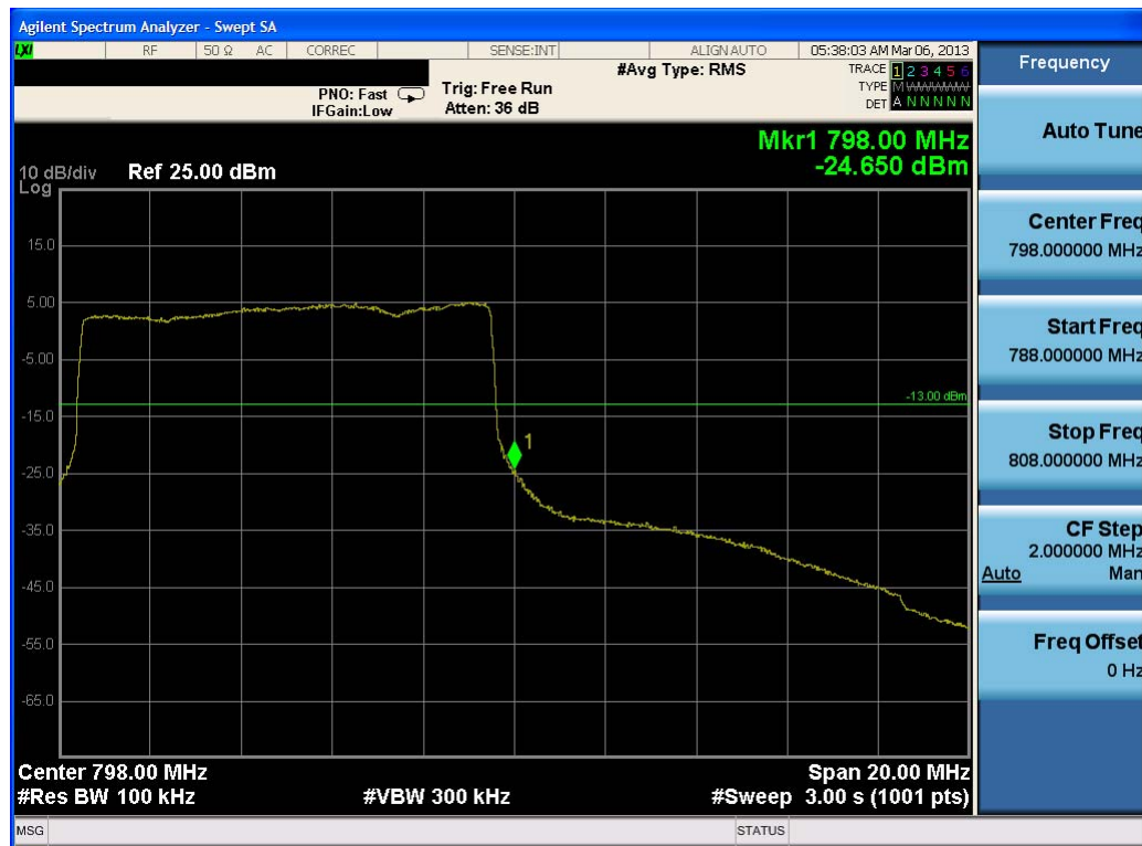
Plot 8-4. Upper Band Edge Plot (16QAM, 50RB)
