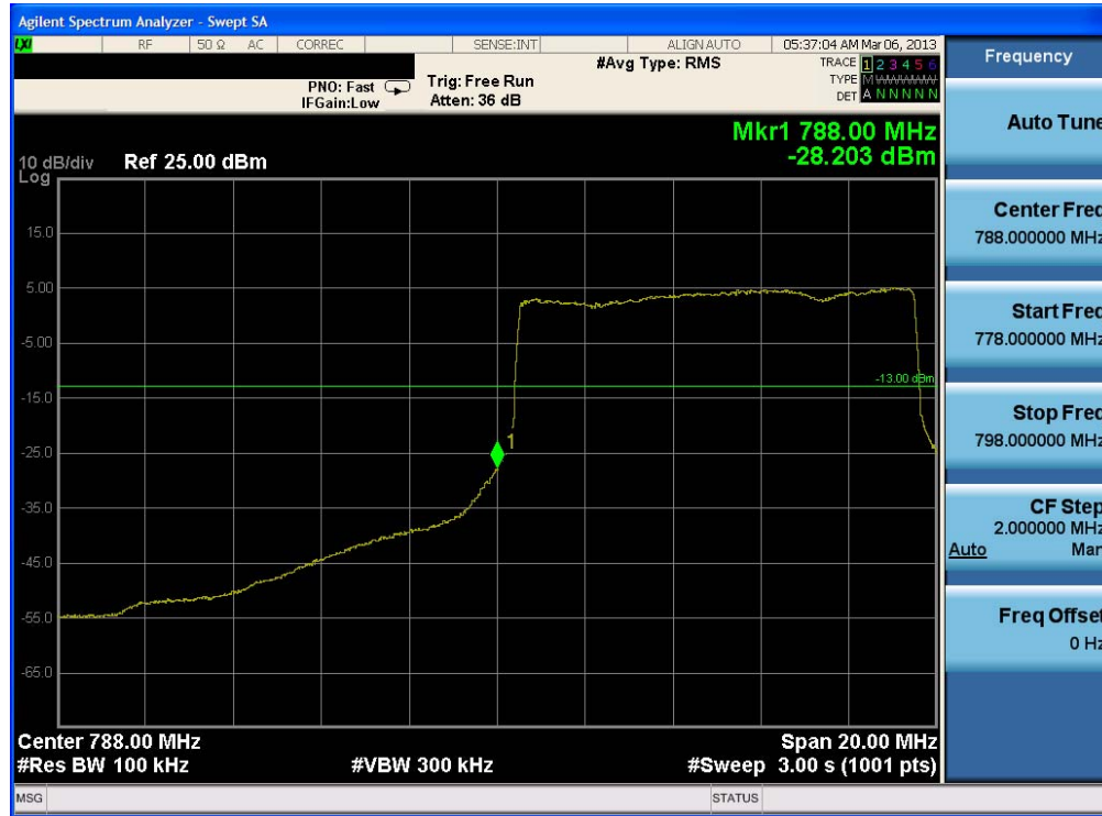
Plot 8-1. Lower Band Edge Plot (QPSK, 50RB)
