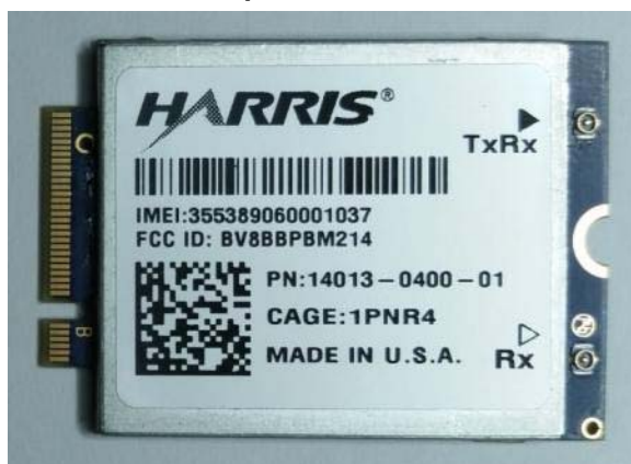
Module topside with shield
