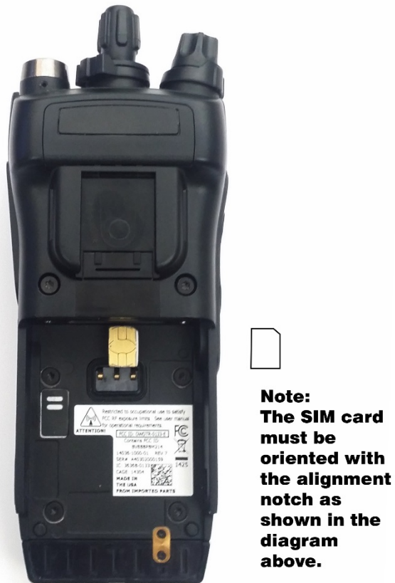
Figure 4-4: SIM Card Installation
