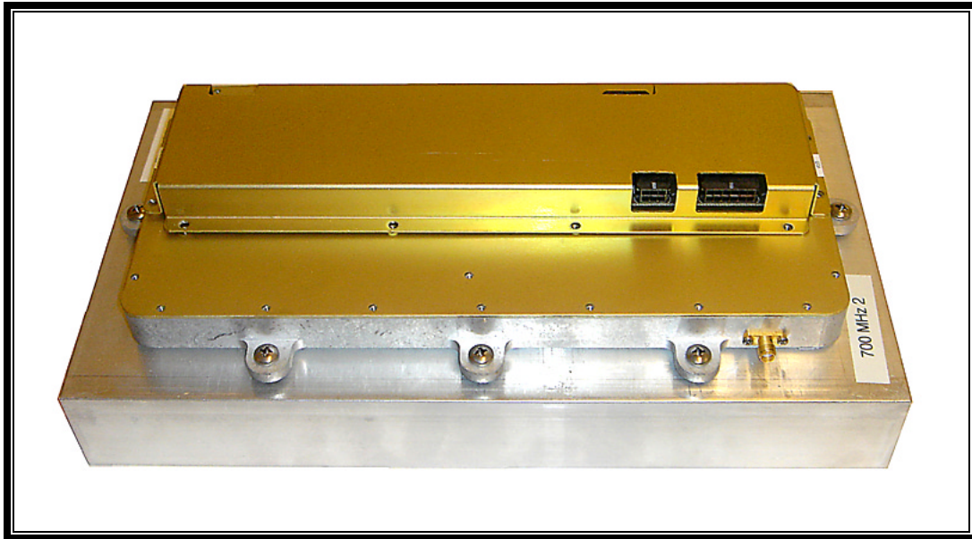
Photograph 15: 700 MHz Cell Site HPA Assembly
