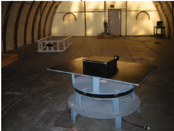
Radiated Spurious Test Setup, Front View
