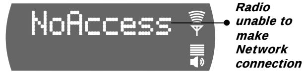
Figure 12 Display Screen—No Access
