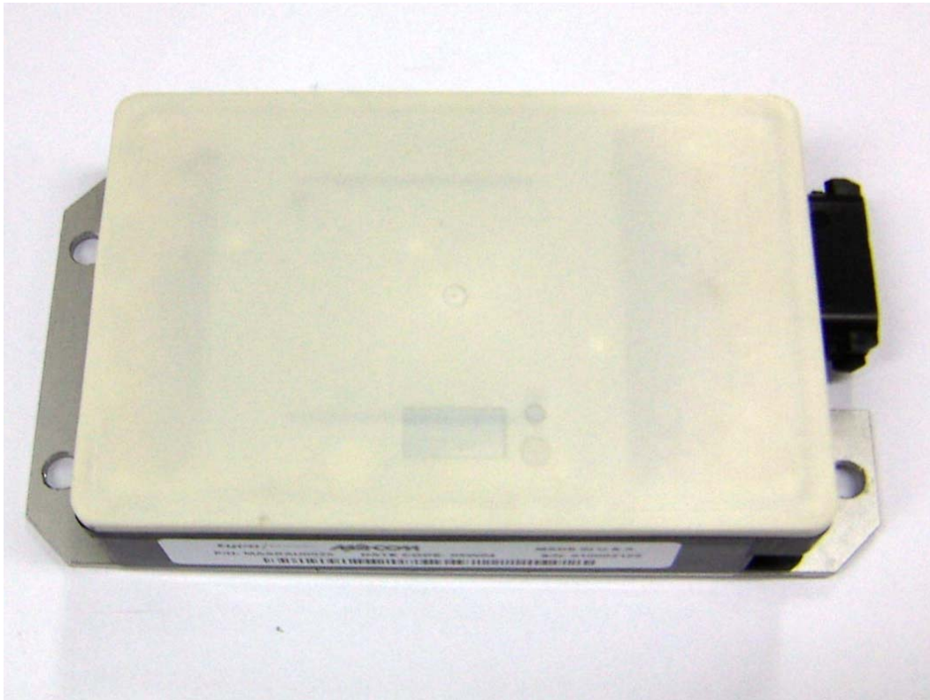
Photograph 3: Front Side View (Sensor Radome Face) of the EUT SN 030002893 (Photo Showing Normal Sensor Orientation)
