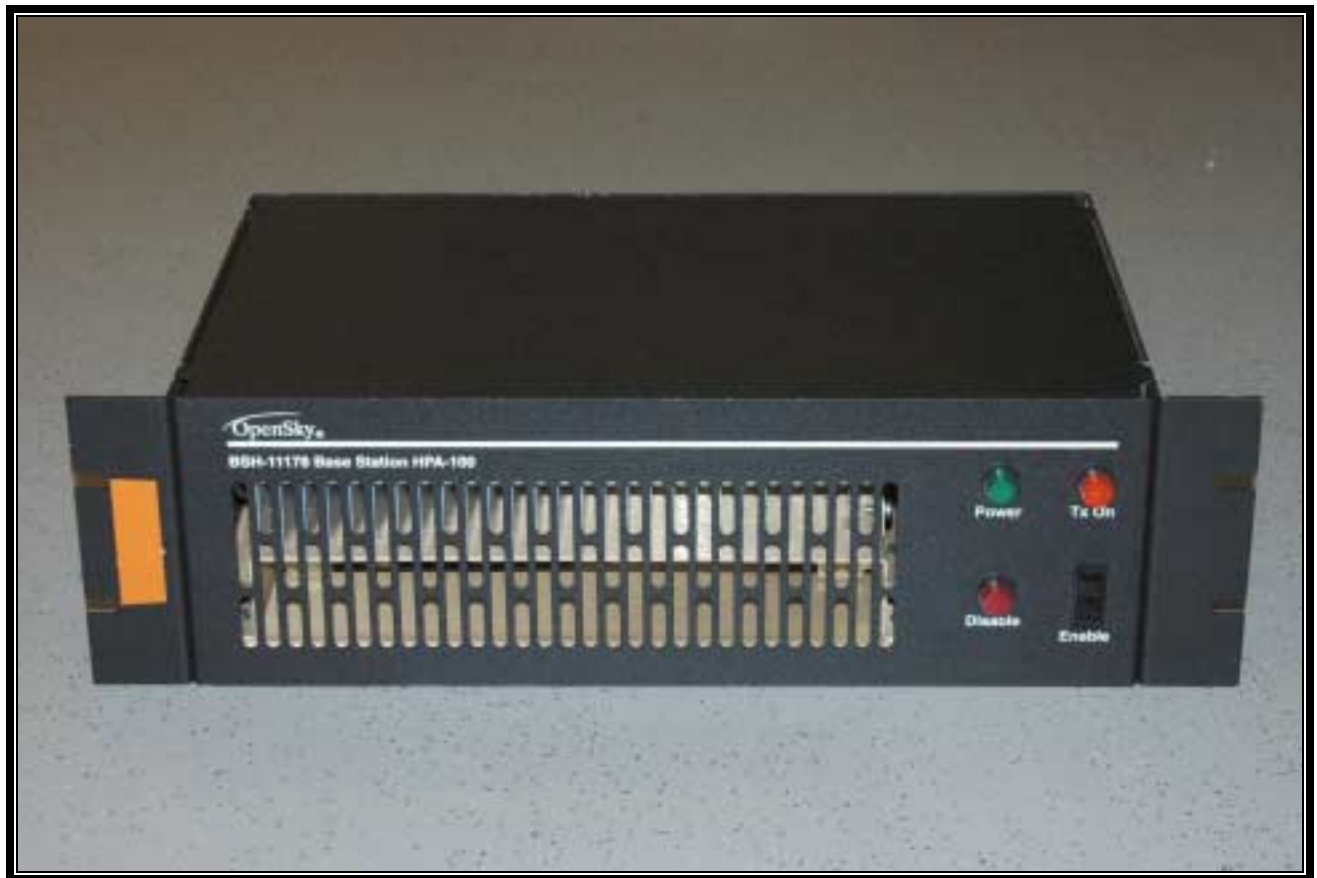
PHOTOGRAPH 6: HPA FRONT VIEW
