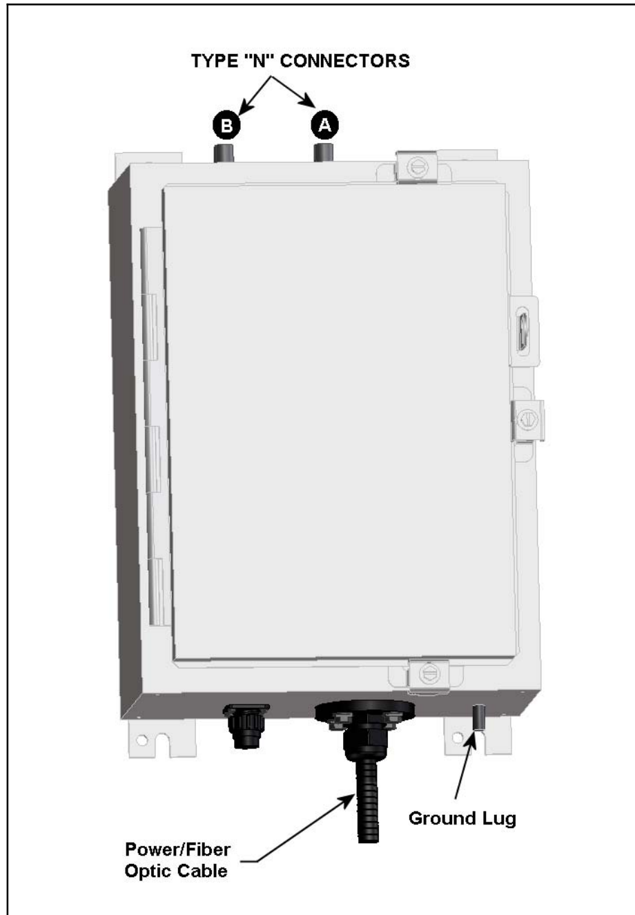
Figure 6-1: ISM Tower Top Radio Enclosure
