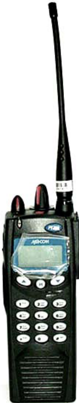
Front of DUT with Half-wave Antenna (P/N: KRE 101 1506/1)
