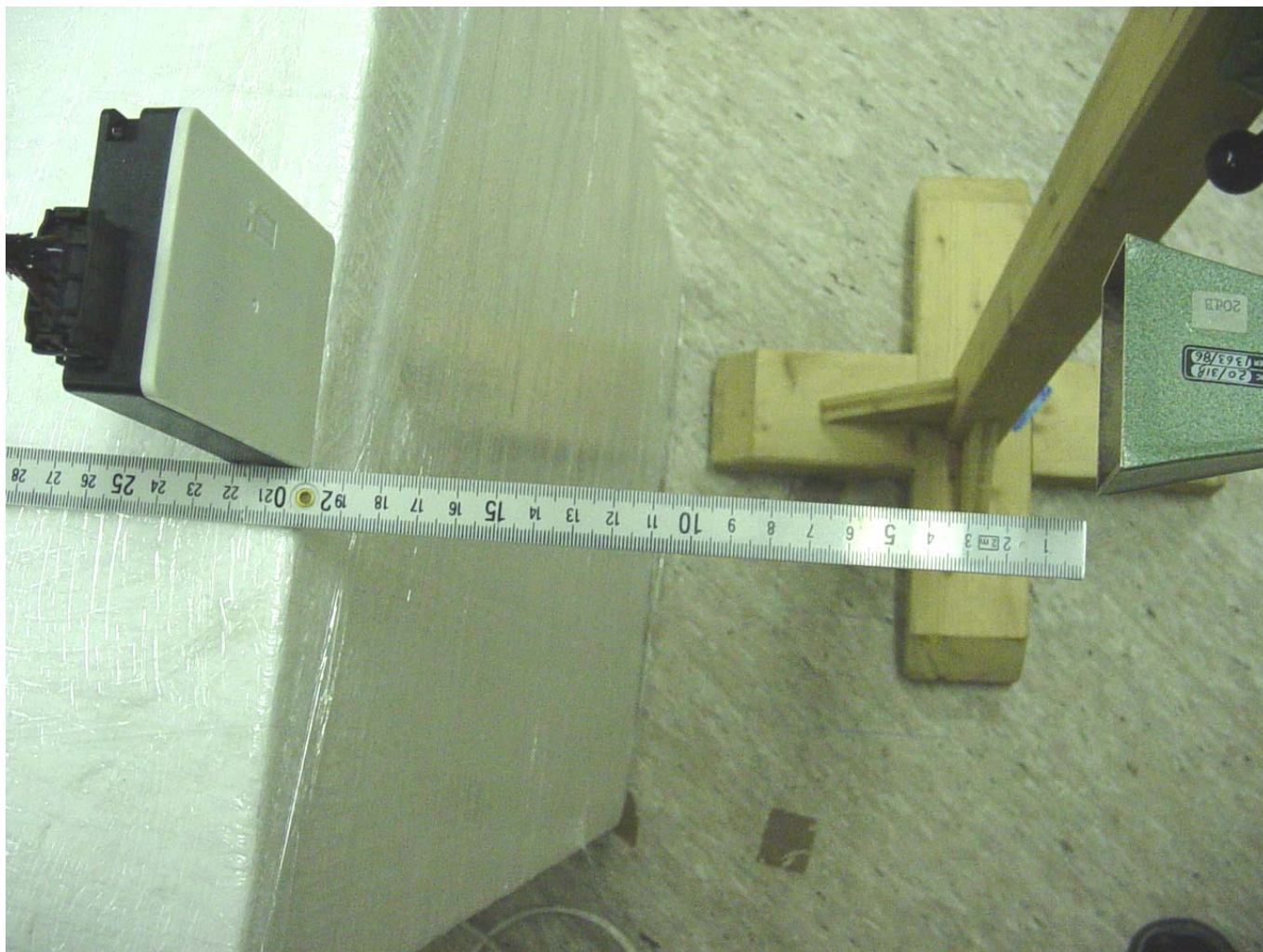
Photograph 5: RF Exposure Measurement at 20 cm Distance
