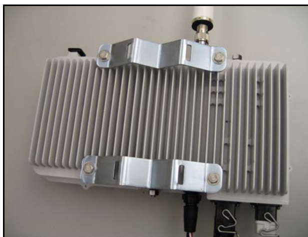
Figure 7-2: Brackets attached to the VIDA MAX Base Station (vertical pole mounting)
