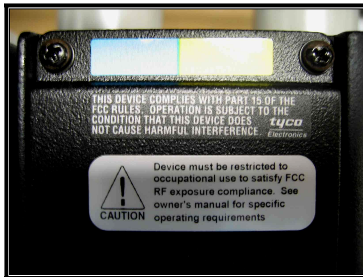
PHOTOGRAPH 2: PART 15 AND RF WARNING LABELS
