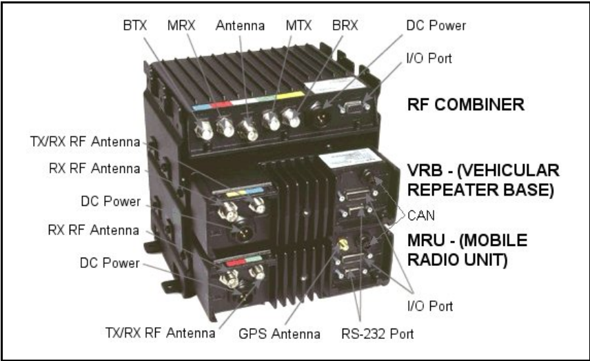
Figure 2-5: V-TAC Rear Panel
