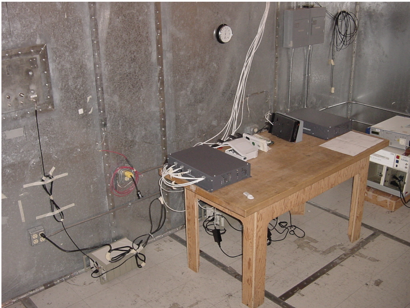
DUT on left corner, accessory layout, antenna cables routed to exit chamber through waveguide.
