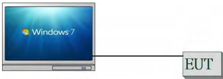
Fig. 2-2 AC Power Line Conducted Emission Configuration
