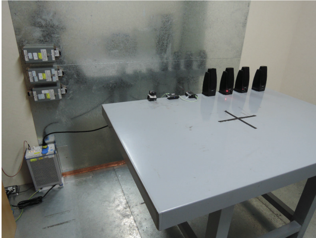
Photograph 6: Set-up for for Mains Conducted testing Front
