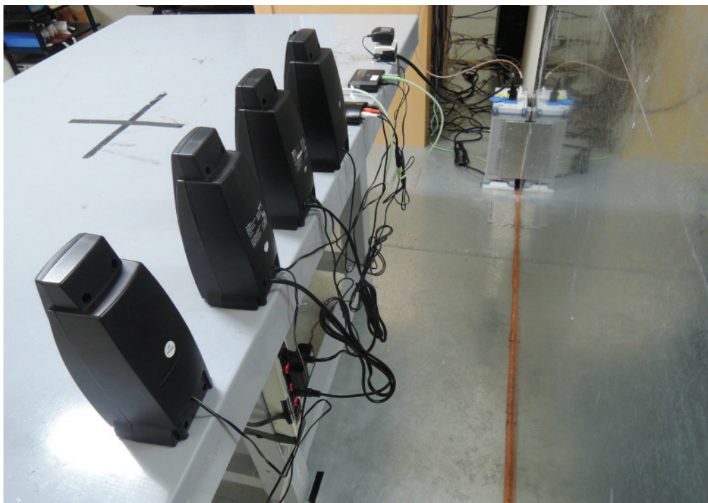
Photograph 5: Set-up for for Mains Conducted testing Back
