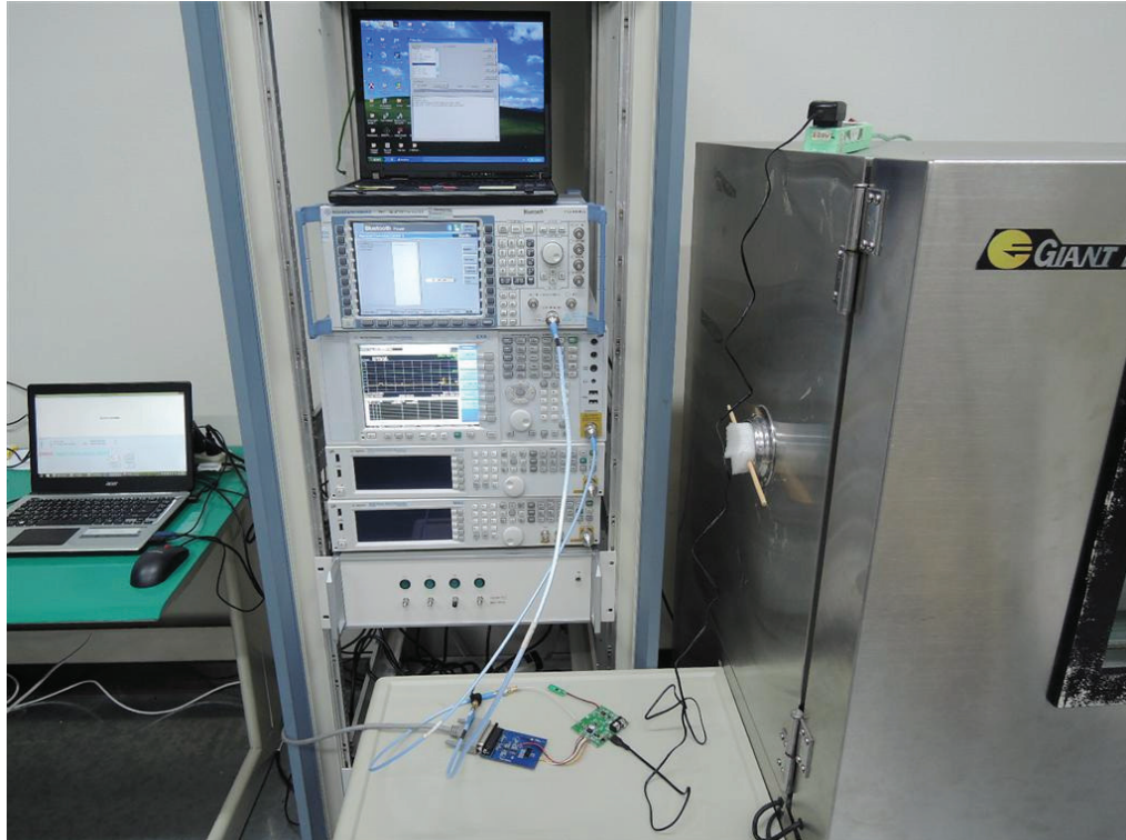
Photograph 4: Set-up for Conducted testing
