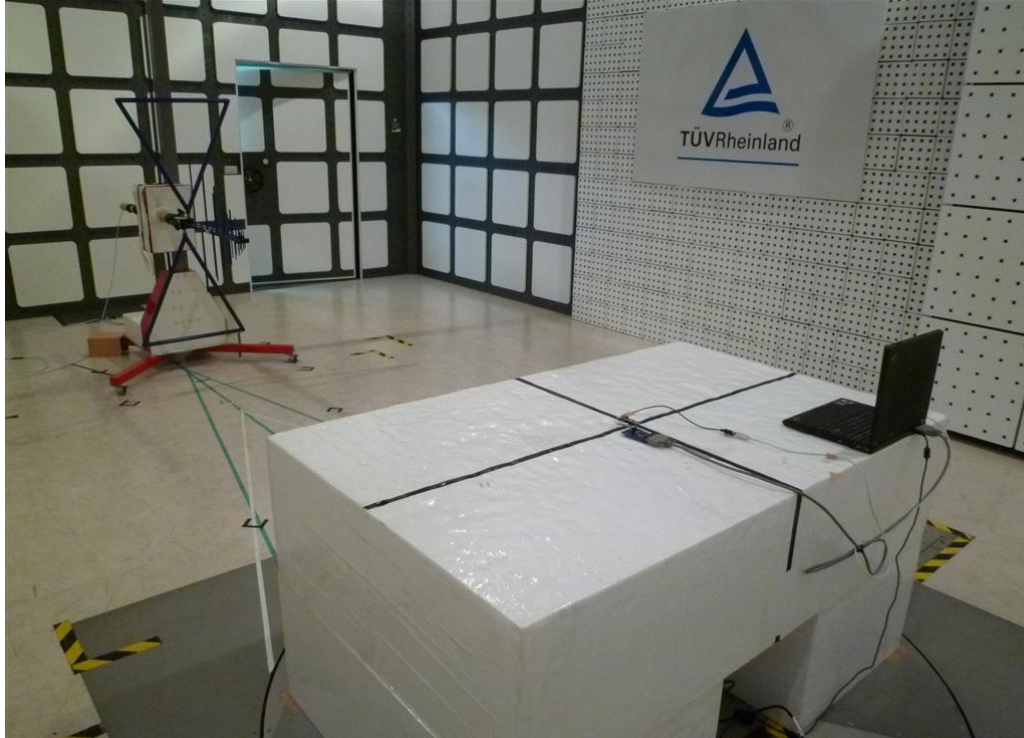
Photograph 2: Set-up for Spurious Emissions (Back View 1)
