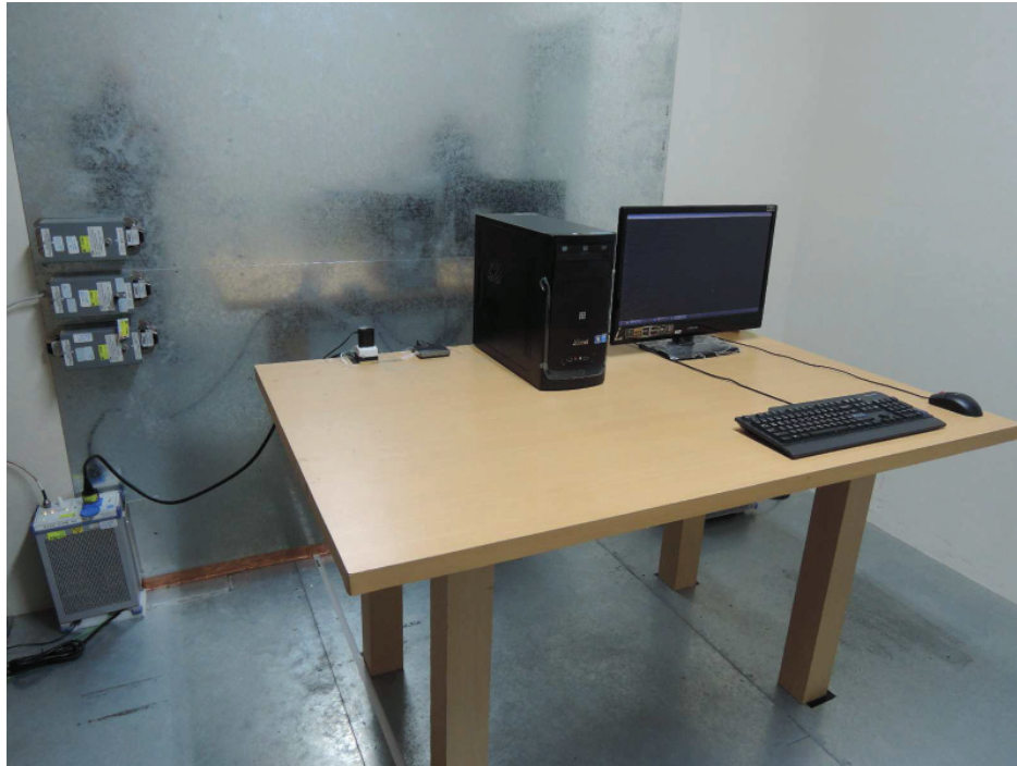
Photograph 6: Set-up for for Mains Conducted testing Front
