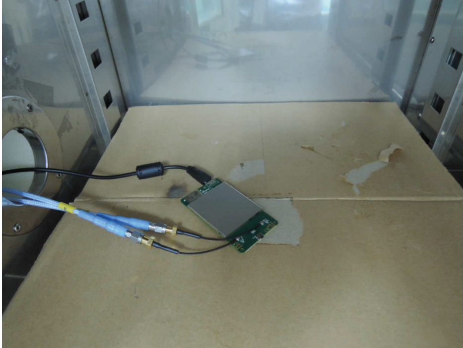
Photograph 4: Set-up for Conducted testing
