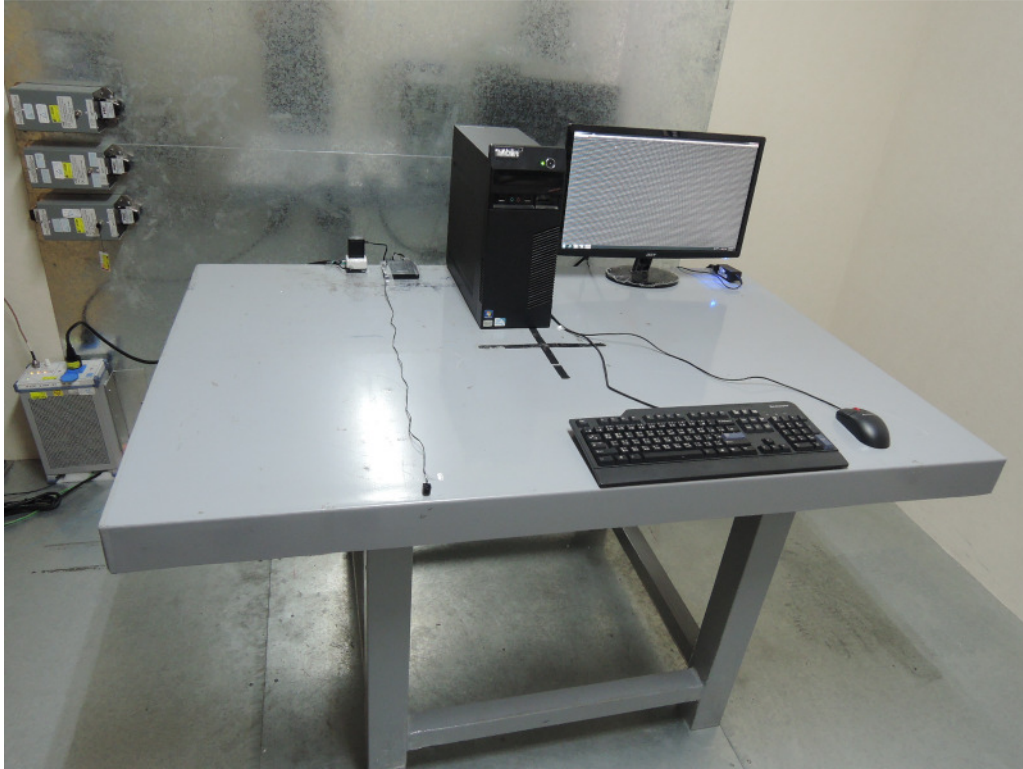
Photograph 6: Set-up for for Mains Conducted testing Front
