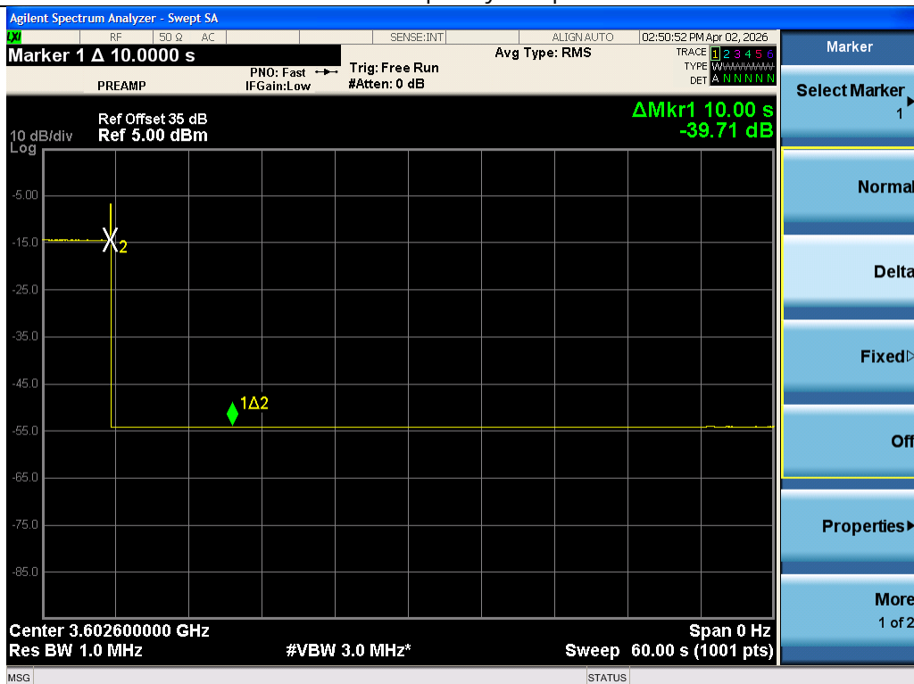
EUT stops transmission within 10 seconds
