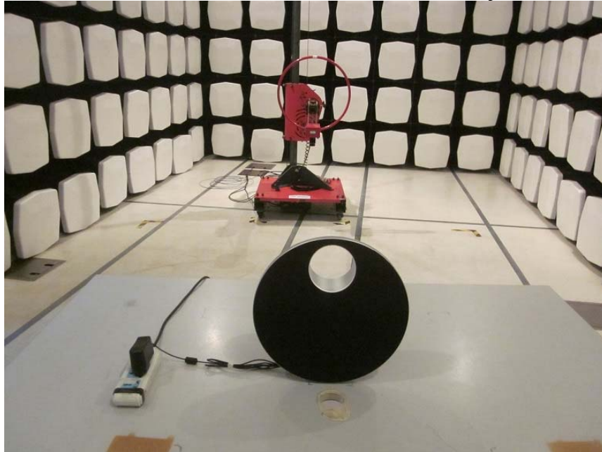
Measurement of Radiated Emission Test Set Up
