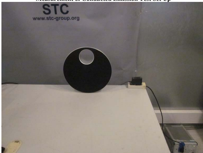
Measurement of Conducted Emission Test Set Up
