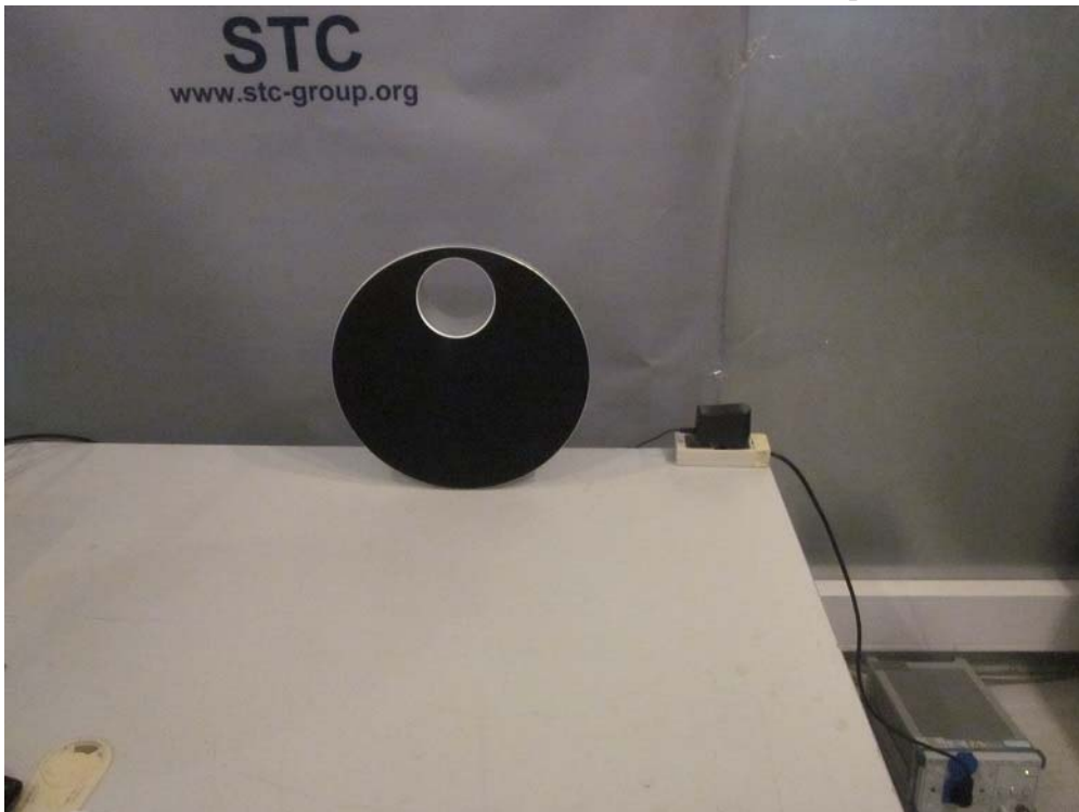
Measurement of Conducted Emission Test Set Up
