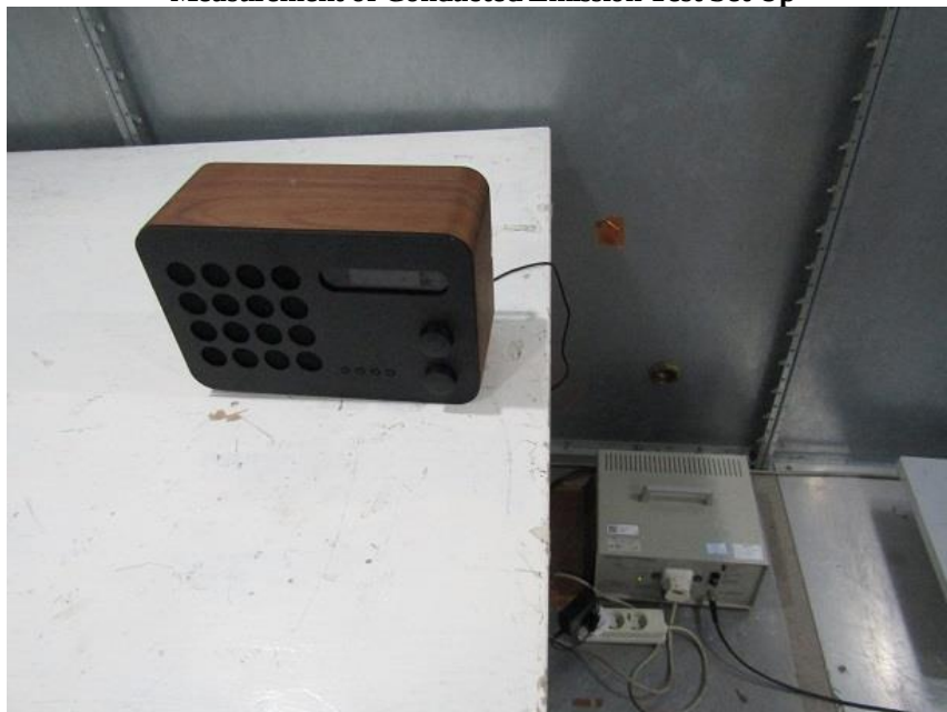
Measurement of Conducted Emission Test Set Up
